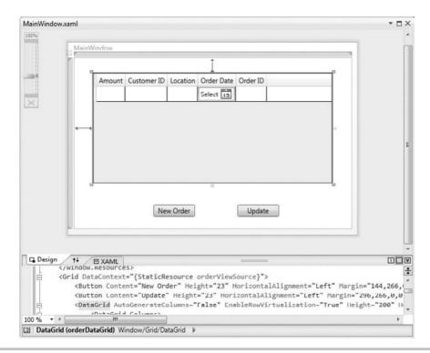
Figure 8-16 Displaying information in a Grid
